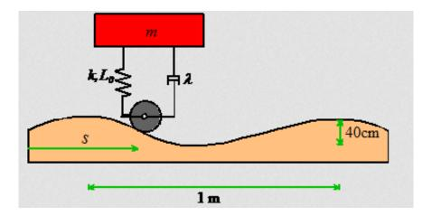
**Solution:** Let s denote the distance travelled by the car and let L denote the wavelength of the bumps and H the bump amplitude". Then the height of the wheel above the mean road height may be expressed as
